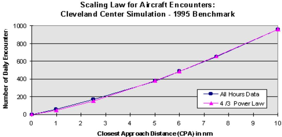
*Figure 5: Power Law Provides Good Fit for Encounters Versus CPA Distance*
