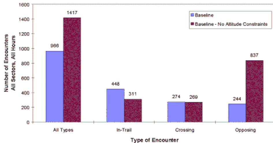
**Figure 4: Effect of No Altitude Constraints**
