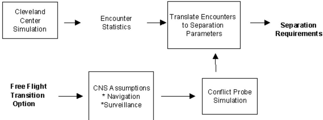
*Figure 1 : Methodology to Obtain Requirements for Free Flight Transitions*
