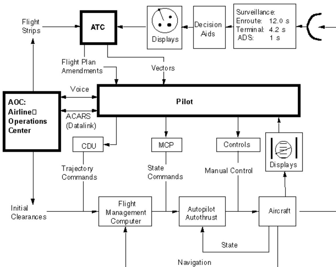
Figure 1. Simple Closed Loop Model of the ATM System.
