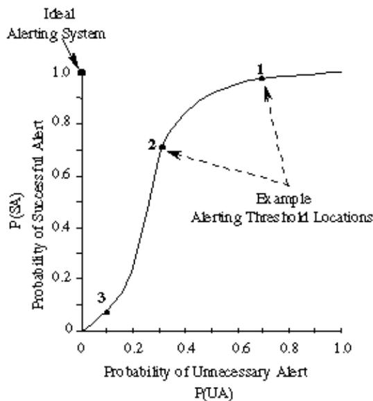
Figure 4. Example System Operating Characteristic Curve.
