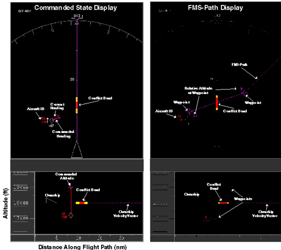
Figure 2. Commanded State and DMS-Path Displays.
