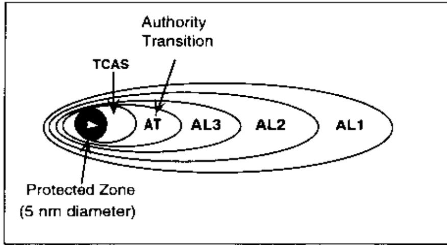
Figure 1. This diagram represents conceptual alert zones surrounding an aircraft (adapted from Yang & Kuchar, 1997)
