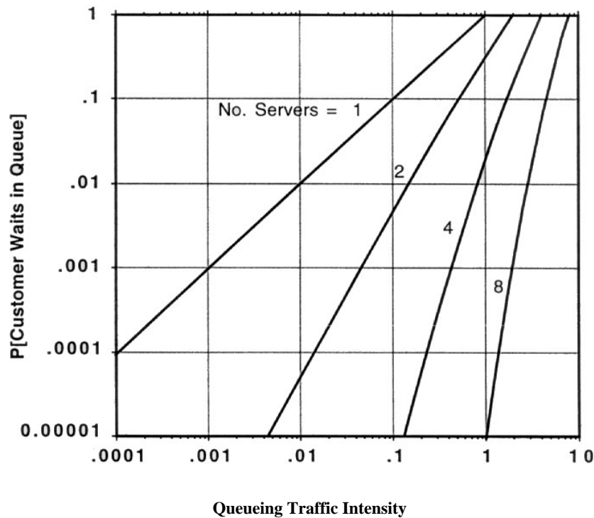
Figure 5.2. The probability that a customer must wait for service is decreased when multiple servers are available.
