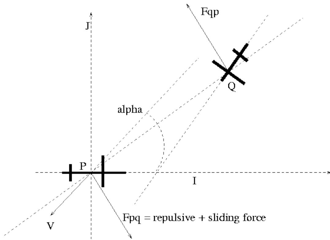
Reactions are applied in the horizontal plane while aircraft are separated, and vertically if they lose separation.
