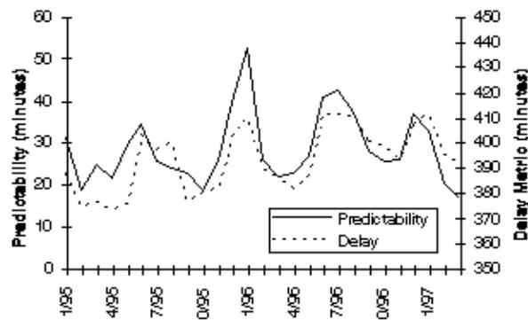
Figure 3. Combined Metrics for the 25 busiest airports: Ground movement delay and predictability
