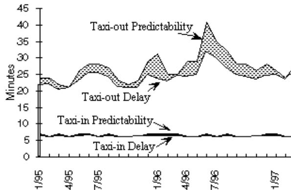
Figure 2. Ground Movement Delay and Predictability for Newark (EWR).
