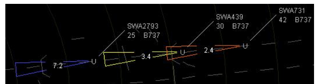
Figure 3. Automated Terminal Proximity Alert
