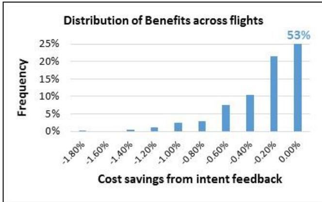
Figure 9. Distribution of cost savings from a base case assuming route-specific historical knowledge across flights due to feedback of ATC Intended route and constraints (53% get no change)
