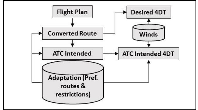
Figure 1. Process for computing Desired and ATC Intended 4DT
