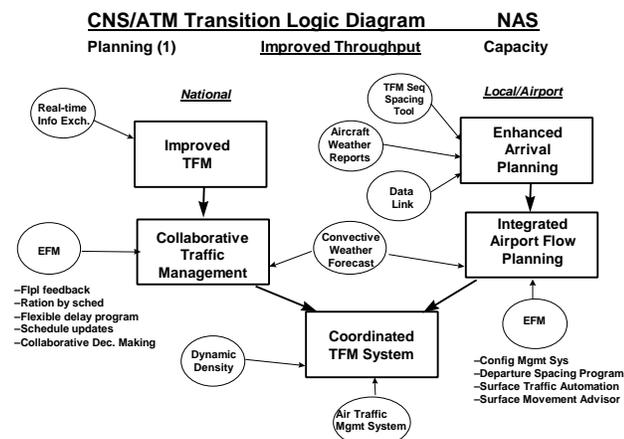
Figure 6. CNS/ATM Transition Logic for Flow Management
