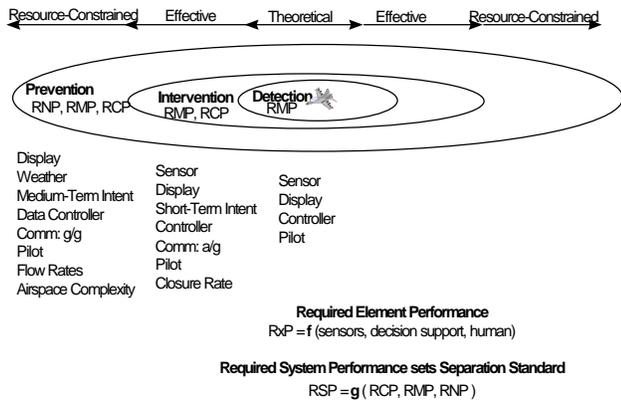
Figure 5. Traffic Spacing and Performance Factors
