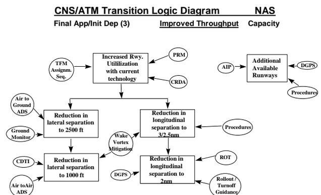
Figure 9. Final Approach and Initial Departure Reduction in Lateral Separation to 2500 ft
