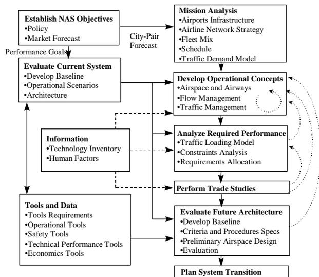
Figure 1. Preliminary Design Process for the NAS
