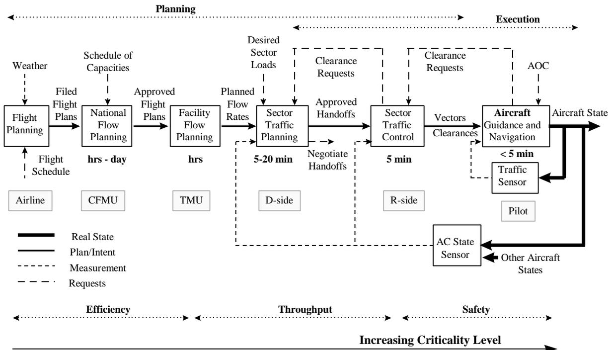
Figure 3. Air Traffic Management System Functional Structure
