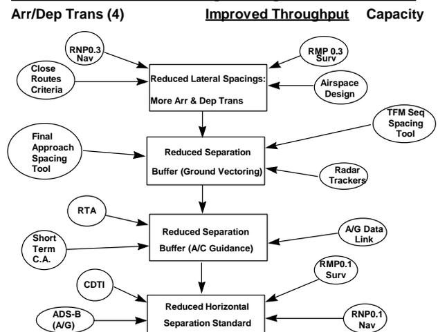
Figure 8. Transition Logic for Arrival Transitions
