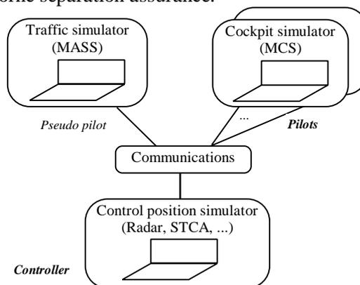
Figure 10: CESAR real-time demonstrator
