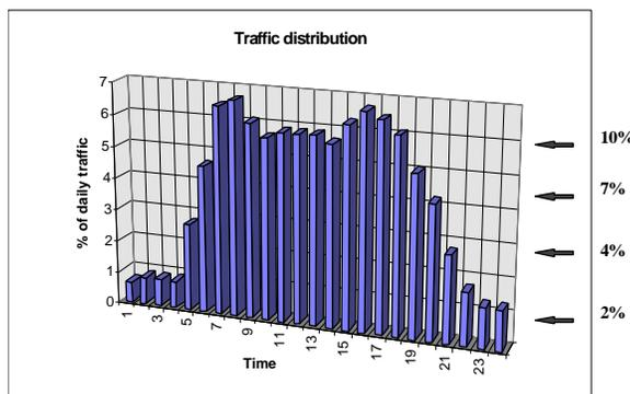
**Figure 2: Trends of Traffic Densities and Their Associated Hourly Weights used in the Simulations.**
