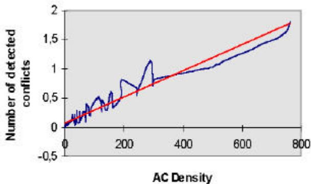
Figure 9 Trends of ADS-B detected conflicts per hour of flight with respect to traffic densities (number of aircraft per hour and per 1MKm<sup>2</sup>).
