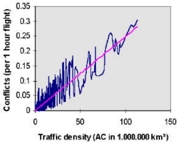
Figure 8 Trends of ADS-B detected conflicts per hour of flight in low-density airspace
