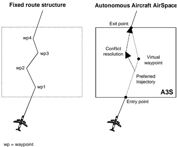
Figure 3 Assumption for Free-Routing
