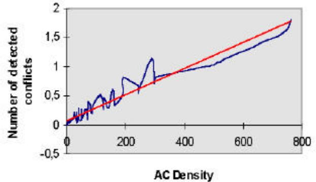
Figure 10 Average number of actively resolved conflict by an aircraft during 1 hour of flight with respect to variations in traffic density
