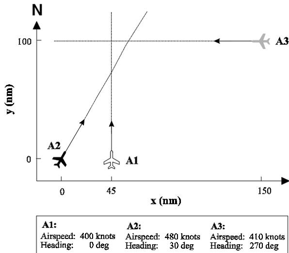
Figure 2. Initial configuration for three aircraft conflict.
