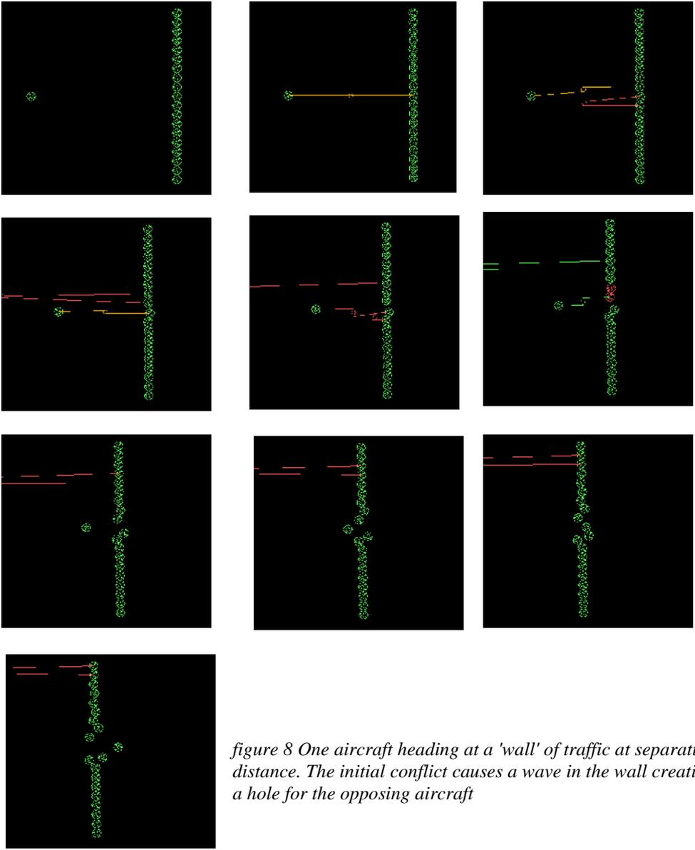
*figure 8 One aircraft heading at a 'wall' of traffic at separation distance. The initial conflict causes a wave in the wall creating a hole for the opposing aircraft*
