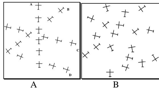
Figure 1 Schematic representation of how airways aid organization of traffic (A=airways, B=direct routing)
