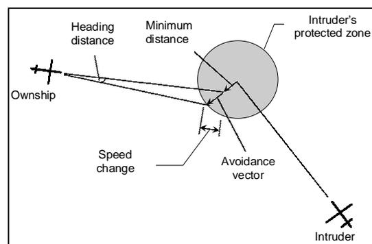
figure 2 Resolution advisory is based on geometry of Closest Point of Approach
