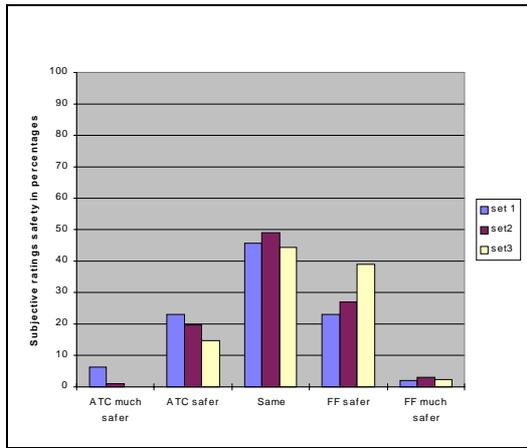
figure 3 Rating of safety by subject pilots in comparison with ATC for each set (1,2 or 3) of 6 runs in the experiment
