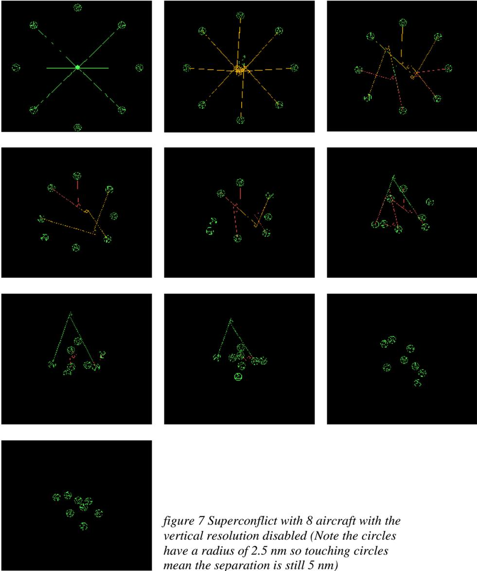
*figure 7 Superconflict with 8 aircraft with the vertical resolution disabled (Note the circles have a radius of 2.5 nm so touching circles mean the separation is still 5 nm)*
