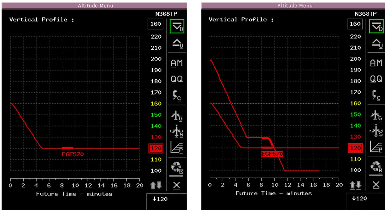
Figure 7. Trial Plan and Conflicting Aircraft Vertical Profile Display
