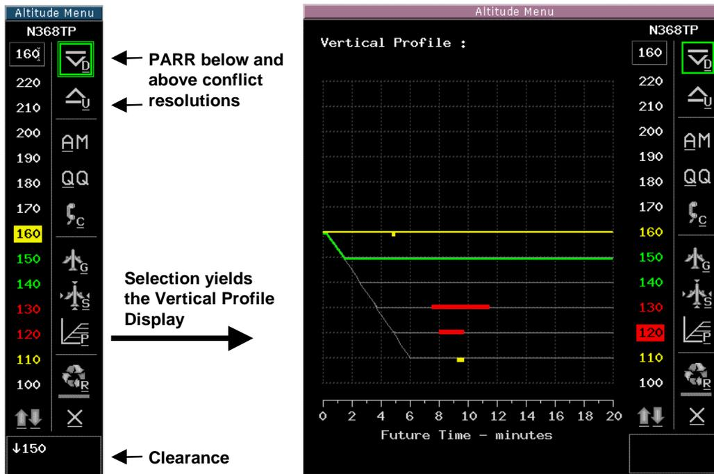
Figure 6. Enhanced Probed Altitude Menu with Vertical Profile Display
