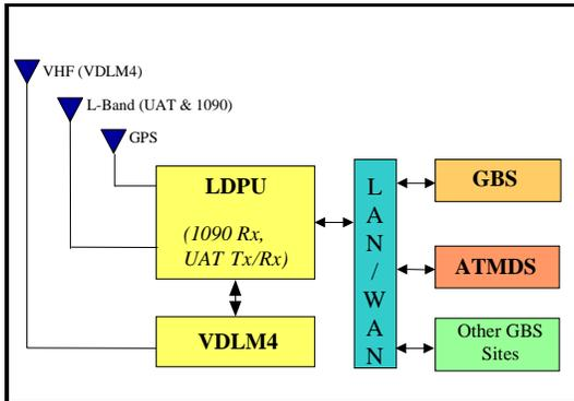
**Figure 2: SF21 ADS-B Ground Station General Architecture**
