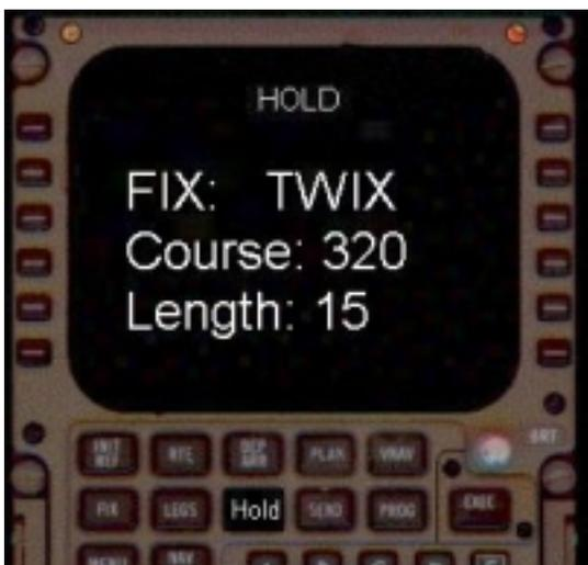
Figure 1a: FMS interface for Holding Pattern
