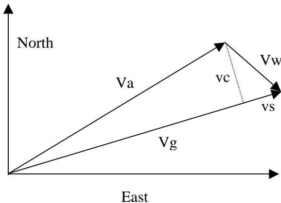
Figure 3: Wind Triangle for Airspeed Vector
