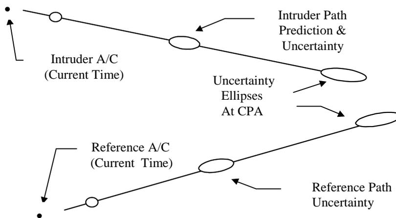
Figure 1: Aircraft Horizontal Prediction Uncertainty (Crossing Path Geometry)
