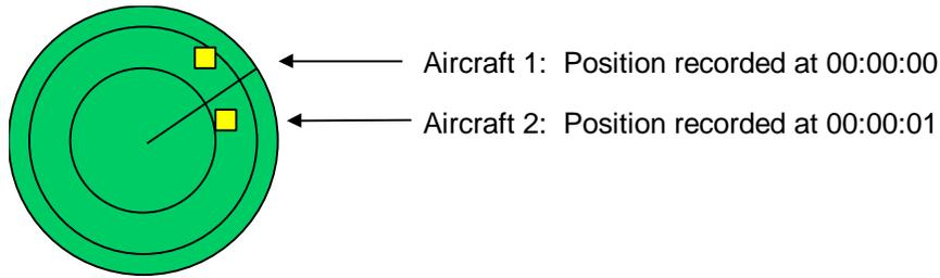
**Figure 7. Radar Aircraft Position Recordings**
