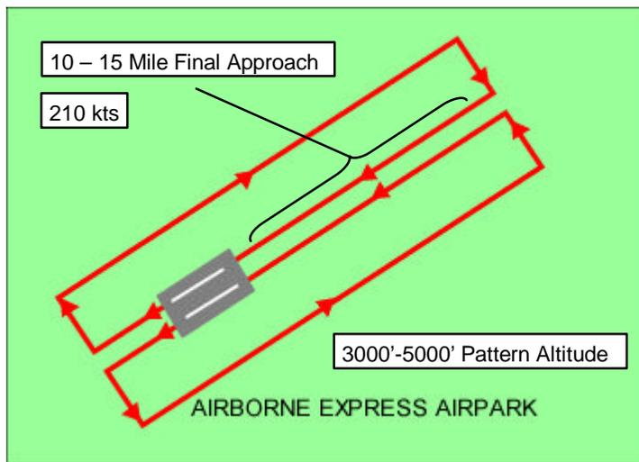
**Figure 1. Flight Profiles**
