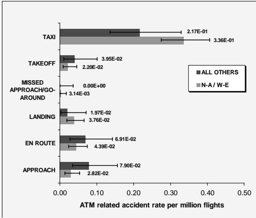
Figure 9: ATM related accident rate by flight phase.
