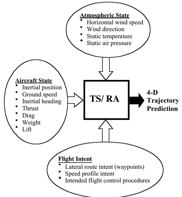
Fig. 1 Inputs to CTAS Trajectory Prediction Process
