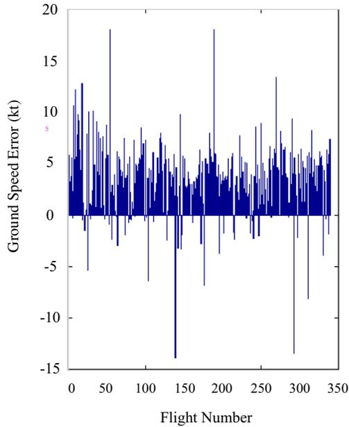
Fig. 3 Signed Error in Mean Ground Speed
