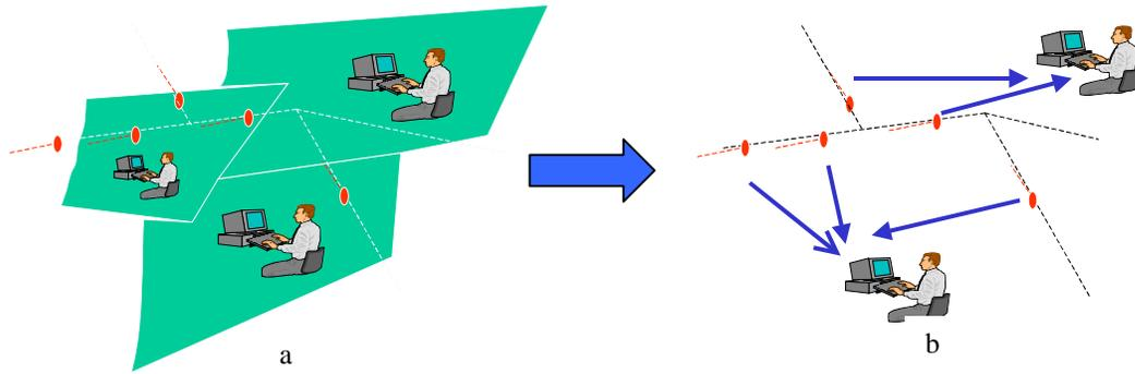
**Figure 1** Basic of Sector-less concept: removing sectors and allocating aircraft to controller for individually management of flight safety. (a) Illustrates current airspace-based ATM with division of airspace into sectors (b) illustrates sector-less ATM concept from which sectors are removed, and controllers manage flight safety individually.
