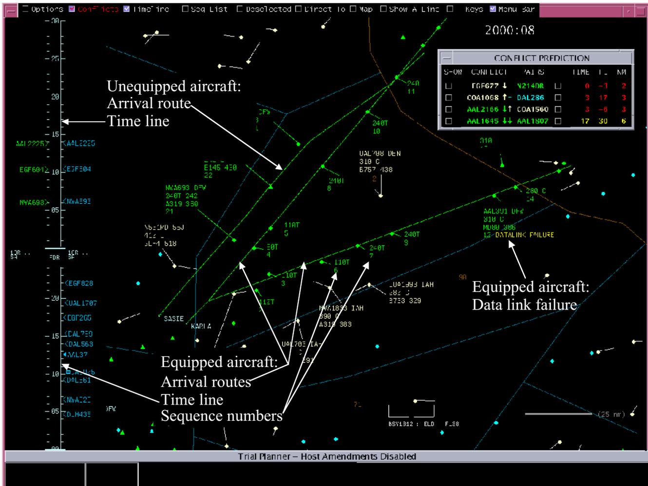
Figure 7; controller display for automated airspace sector
