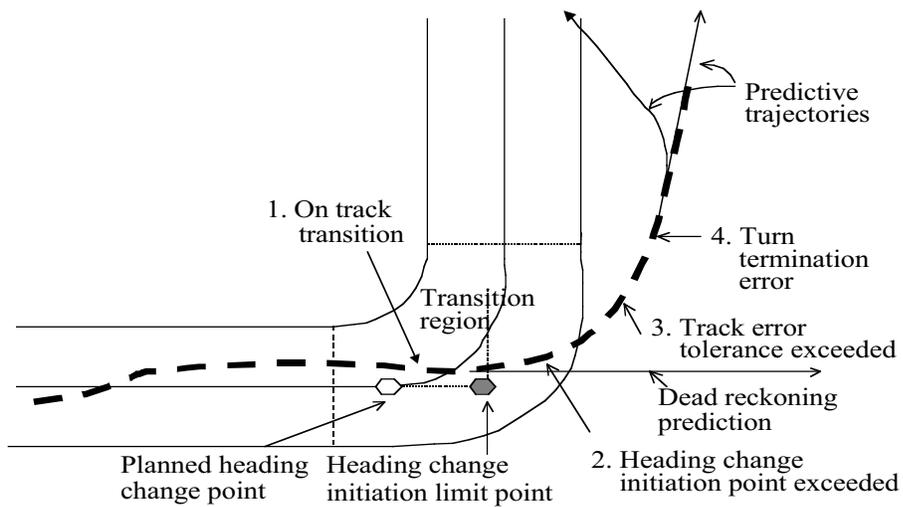
Figure 5: Illustration of Horizontal Transition Errors
