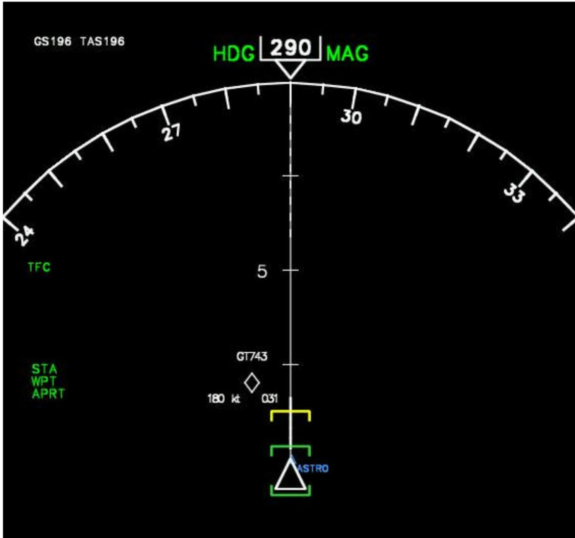
Figure 9. Navigation display with indication of parallel traffic, actual safe zone and predicted safe zone
