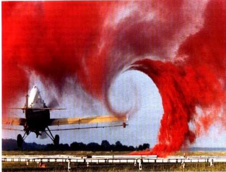
Picture 1. Visualisation of a Wake Vortex thanks to coloured smoke.
