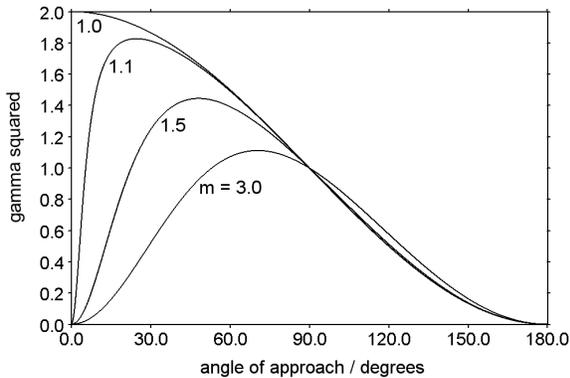
**Figure 4: Minimum displacement variance against angle of approach for various ratios of speed**
