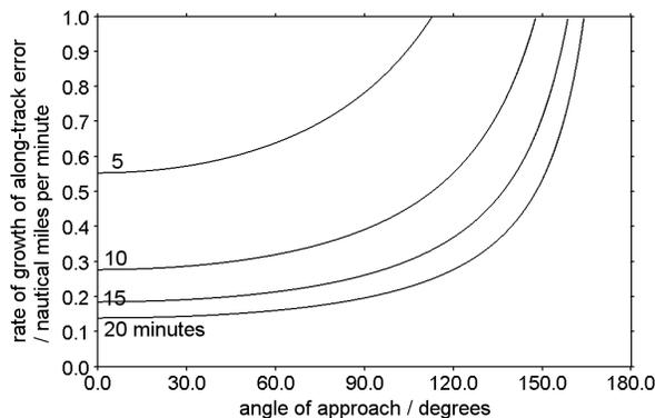
**Figure 13: Required rate of growth of along-track error**
