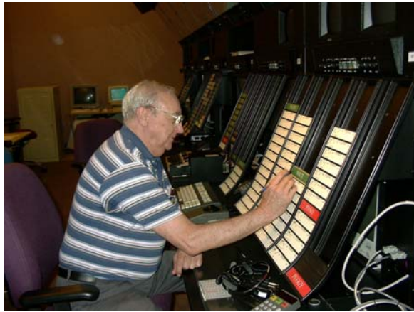
Figure 16: Oceanic controllers assure separation using flight strips without aid from a situation display in U.S. facilities. (Photo from Anchorage Oceanic Facility)
