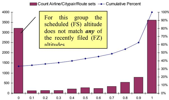
**Figure 1: ETMS sets the FS altitude as the mean of the previous week’s FZ altitudes for each airline/city pair/route combination. This figure shows the fraction of previous week’s FZ altitudes that actually match the current FS altitude (FS date = 5/24/2002, FZ range = 5/16/2002 – 5/22/2002, observed change date = 5/23/2002 ~12:00).**
