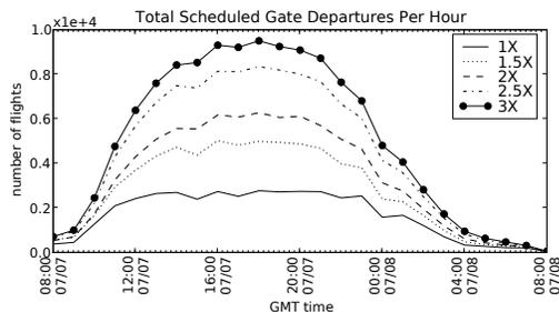
**Figure 4: Departure demand profiles for 1x, 1.5x, 2x, 2.5x, and 3x homogeneous growth based on 7/7/2006 traffic.**
