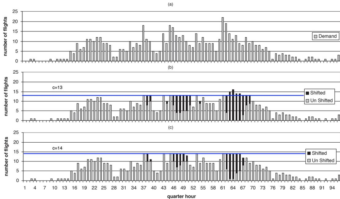
**Figure 3: Required capacity estimation example with a maximum delay per flight of 15 minutes and a maximum average flight delay across the facility of 3 minutes. (a) Demand profile. (b) Unshifted flights and shifted flights for a test capacity of 13 flights. (c) Unshifted flights and shifted flights for test a capacity of 14 flights.**
