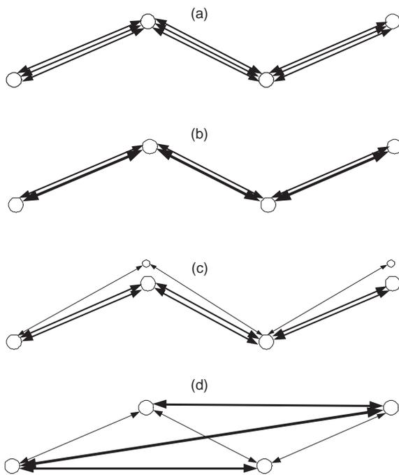
**Figure 8: Business model examples. (a) 3x growth of current traffic. (b) Flight consolidation merges several flights into fewer flights using larger aircraft. (c) PTP-A shifts some flights to satellite airports with smaller aircraft. (d) PTP-B uses larger aircraft to shift to some non-stop flights.**
