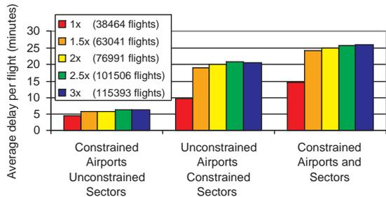
**Figure 6: Average total delay per flight for each of the 5 demands with just airport, just sector, and both airport and sector required capacity constraints.**
