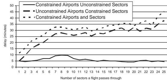
**Figure 7: Average total delay per flight segregated by the number of sectors through which a flight passes for the 3x simulations.**
