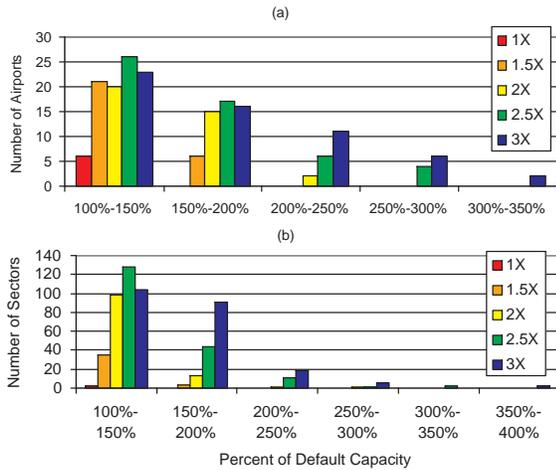
**Figure 5: Required capacity comparisons for 1x, 1.5x, 2x, 2.5x, and 3x. (a) Comparison between number of airports in various ranges of default capacity percentage. (b) Comparison between number of sectors in various ranges of default capacity percentage.**
