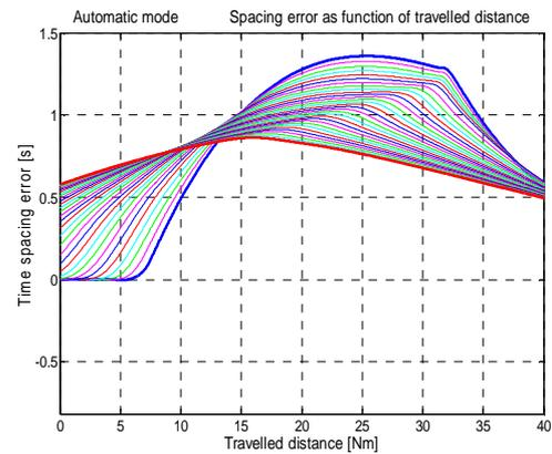
**Figure 5** Continuous time spacing error versus distance, spacing anticipation = 20s, first pair (bold blue), last pair (bold red)
