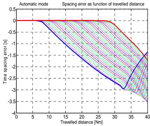
**Figure 3** Continuous time spacing error versus distance, spacing anticipation = 0s, first pair (bold blue), last pair (bold red)
