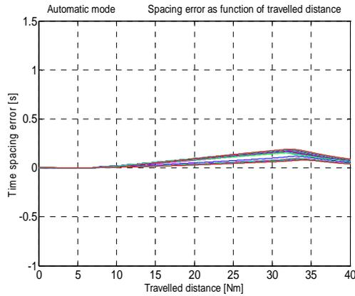
**Figure 4** Continuous time spacing error versus distance, spacing anticipation = 10s, first pair (bold blue), last pair (bold red)
