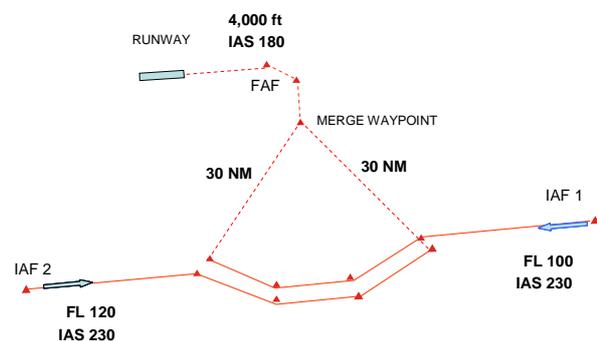
**Figure 2** TMA route structure for merging two traffic streams at a waypoint in descent from IAF to FAF
