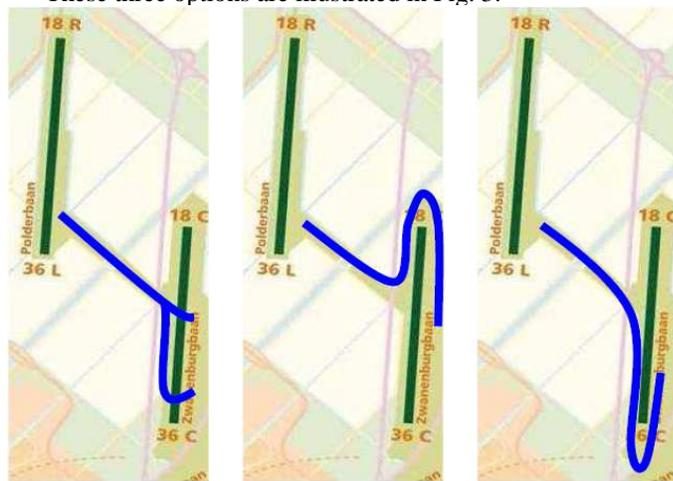
Figure 3. Schematic representation (in blue) of three main development options identified in an early stage: active runway crossings, NTW and STW.
