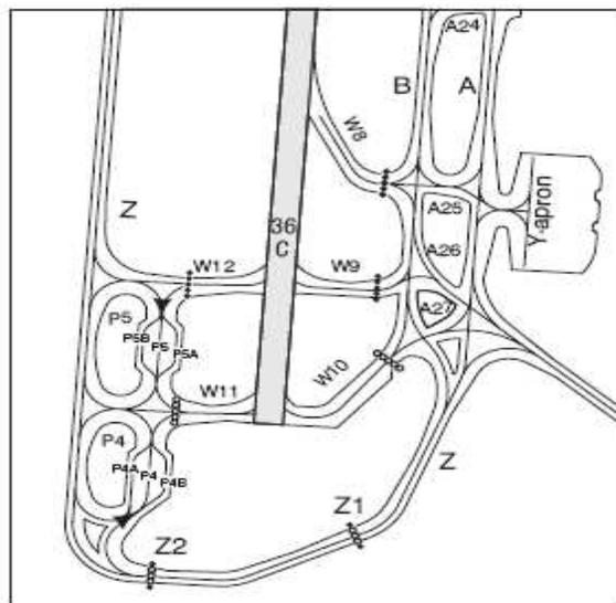
Figure 9. Detail of the infrastructure for dependent taxiing operations on the STW with stop bars at Z1 and Z2.
