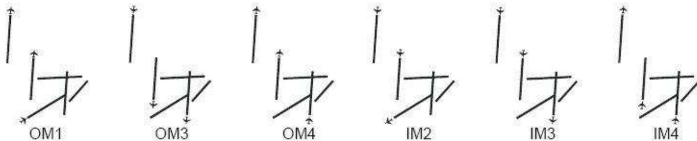
Figure 2. Schematic presentation of the most relevant configuration modes with simultaneous use of runways 18R/36L and 18C/36C.
