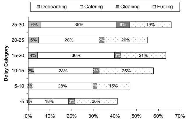
Figure 13. Processes on Critical Path
