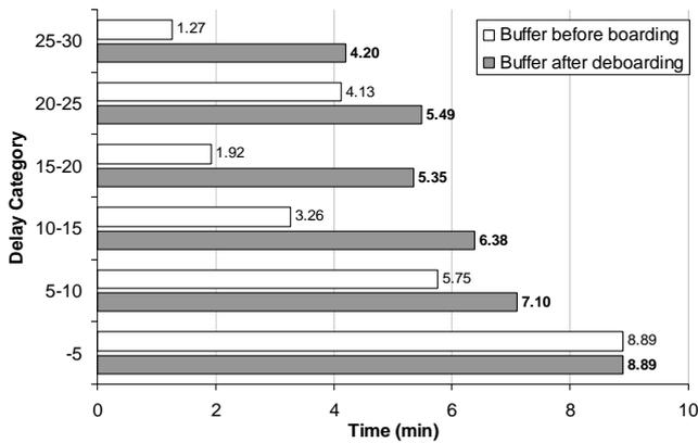
Figure 14. Derived Time Buffer Size for Turnarounds
