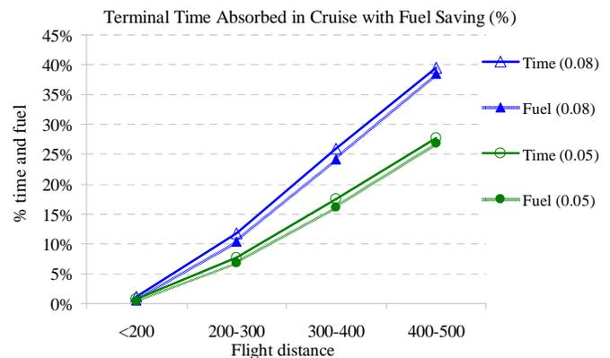
Figure 18. Fuel savings from speed control versus flight length (Europe 2009)
