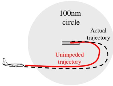
Figure 4. Illustration of excess distance in the descend phase
