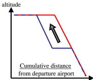
Figure 2. Shifting Level Segment to Cruise – Distance Perspective
